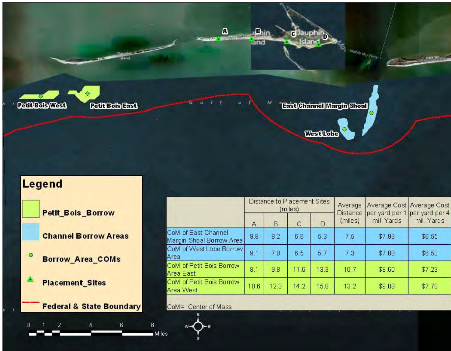
Figure 19. Dredging Cost Estimate. Green dots are centers of mass for the borrow areas and the green triangles are estimated placement sites. Distances are measured from each center of mass to each placement site.
