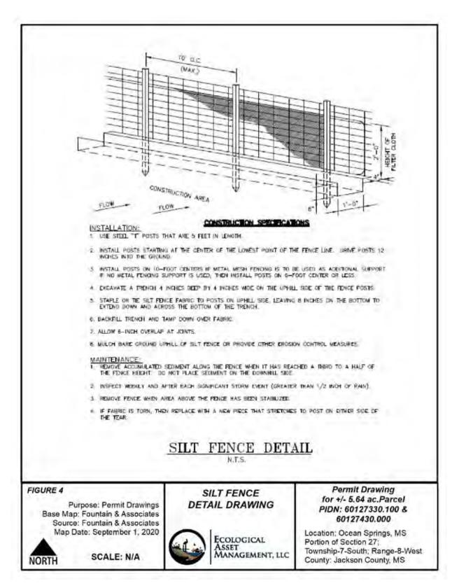
Figure 4: Silt Fence Detail Drawing
