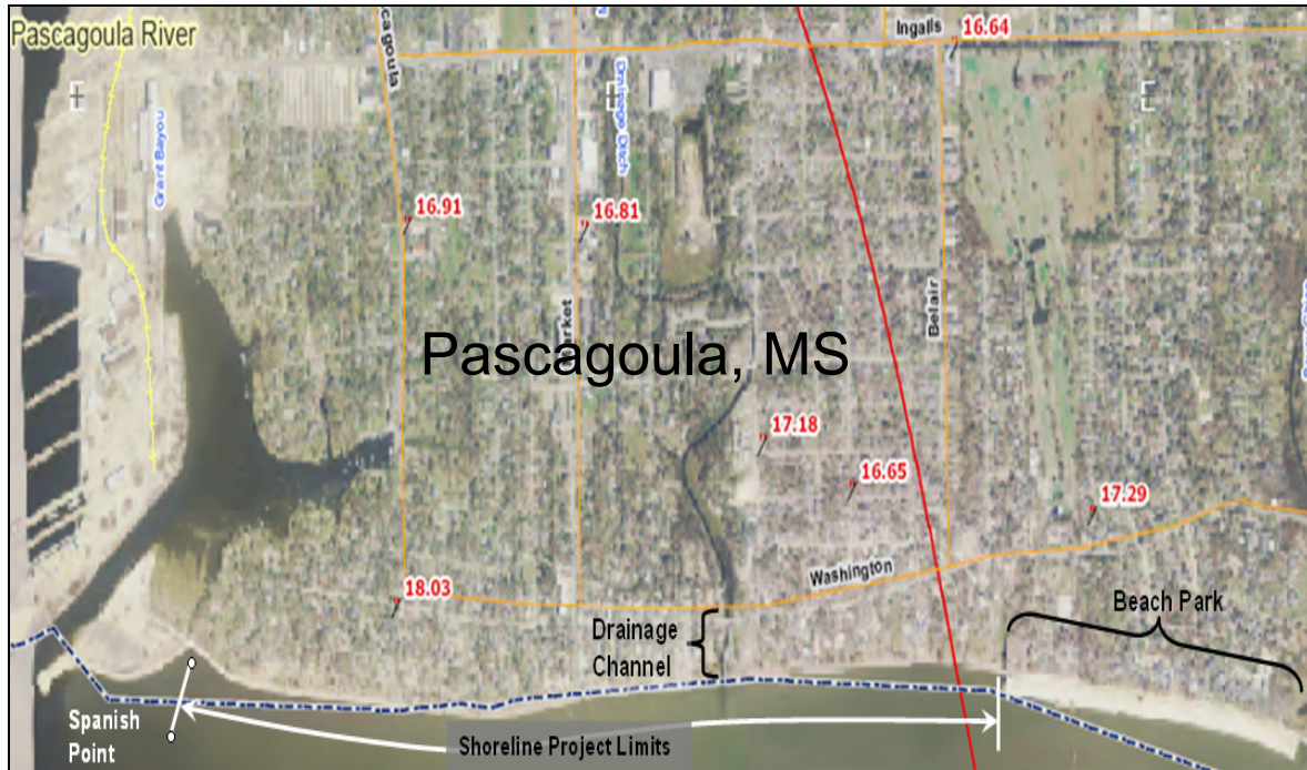
Figure 2.3.13-3. Pascagoula Shoreline West from the East End of Beach Park. Hurricane Katrina High Water Marks in Feet NAVD 88 Datum Shown in Red
