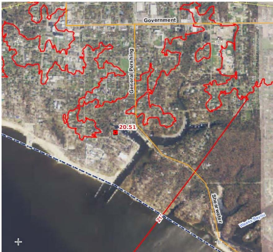
Figure 10. Shearwater Bridge Inundation Limits and 21-ft. Contour
