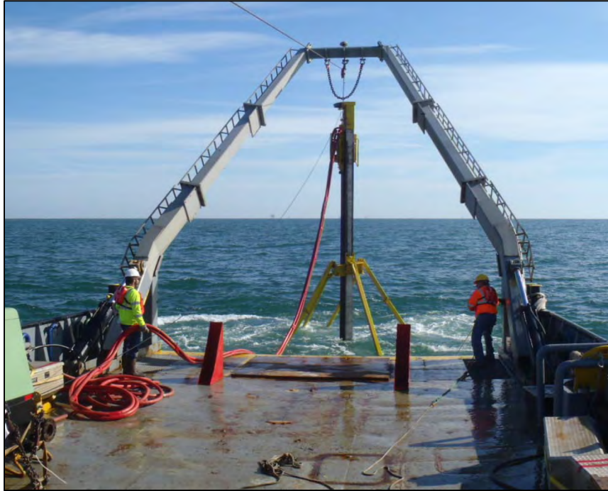
Figure 5.1.2 Vibracore unit being deployed during the 2012 sampling event.
