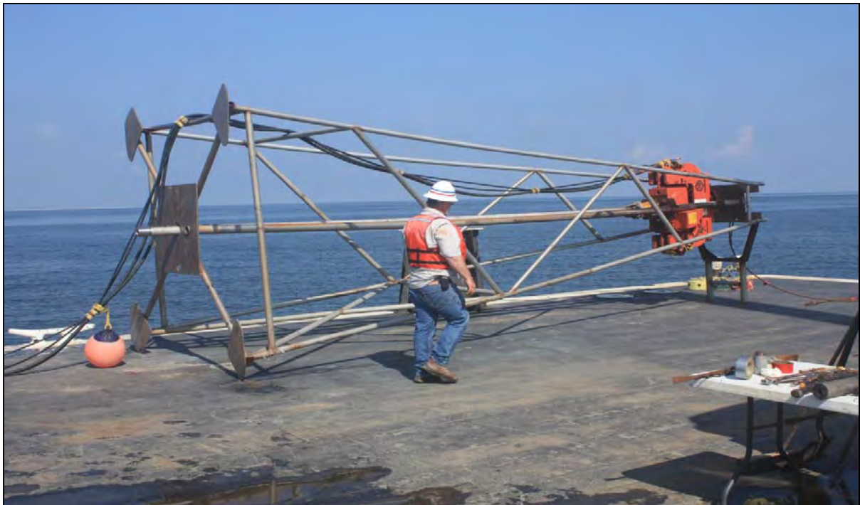
Figure 5.1.1 Vibracore unit used for 2010, 2011, and 2013 sampling events.
