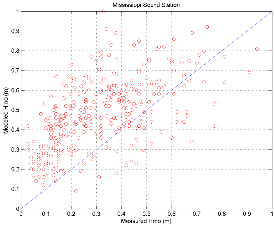
Figure 2-9. Measured vs. Modeled Hmo (m) at the Mississippi Sound Station.
