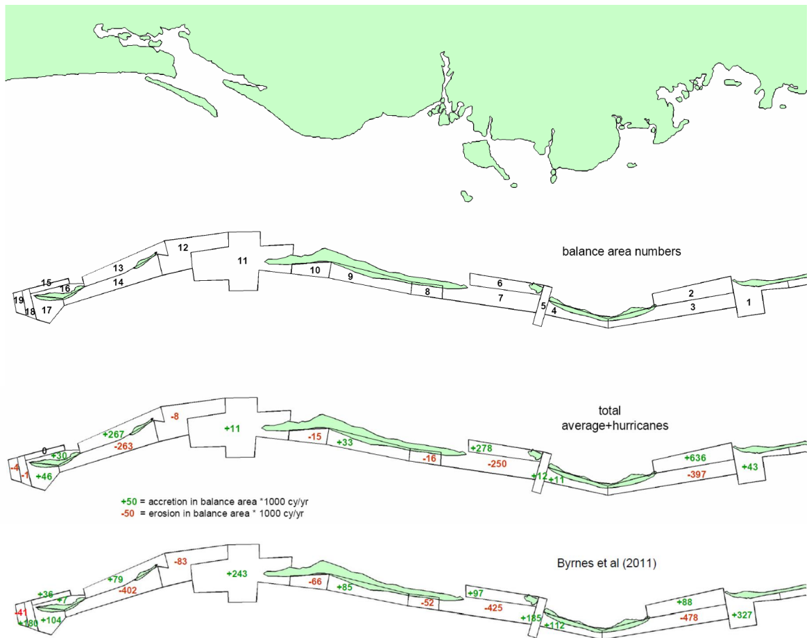
Figure 7.6 Comparison of detailed sediment balance MCC model and Byrnes et al (2011) (Byrnes volumes in areas 5, 18 and 19 have been corrected to account for sand dredging and placement)
