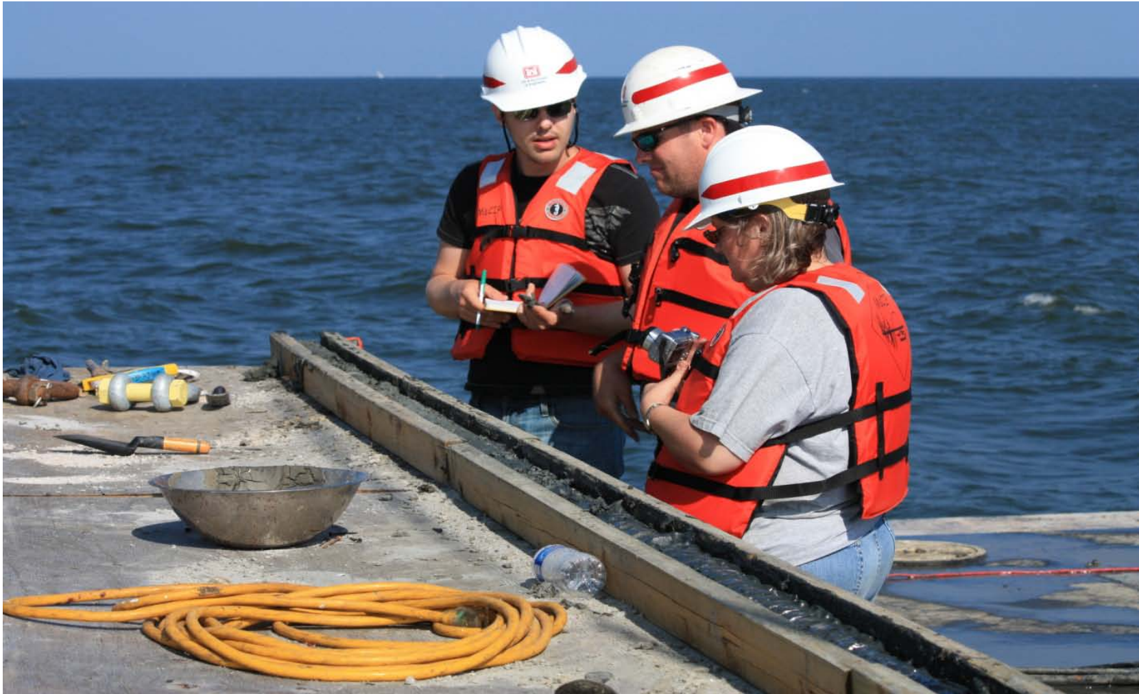
Figure 5.1.4 – Personnel for the USACE and the NPS inspect and log the sample after the inner sleeve is cut open.
