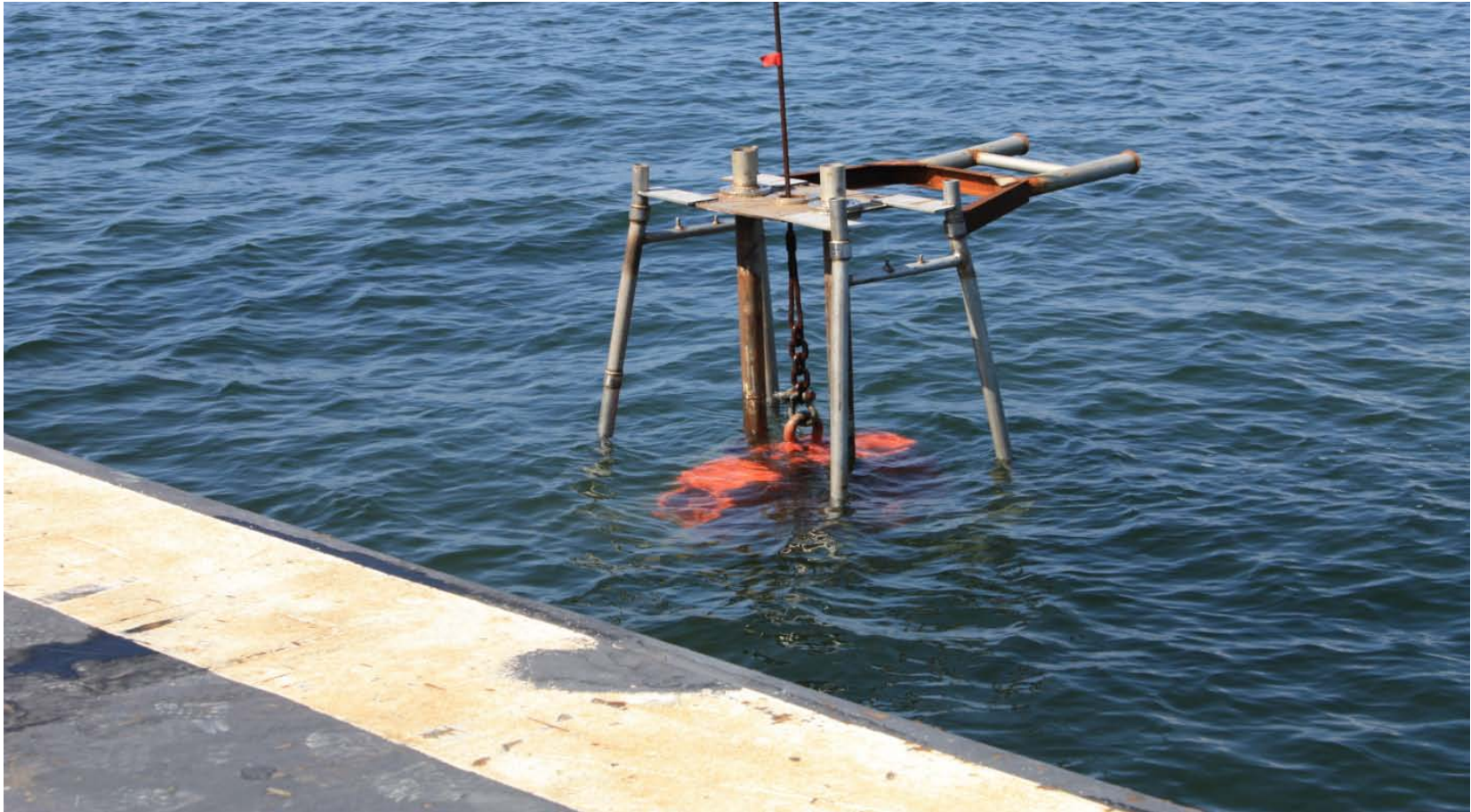
Figure 5.1.2 – VibraCore sampler has been lowered to the bottom and the vibratory unit is activated to push the sample tube into the upper 20 feet of sediment
