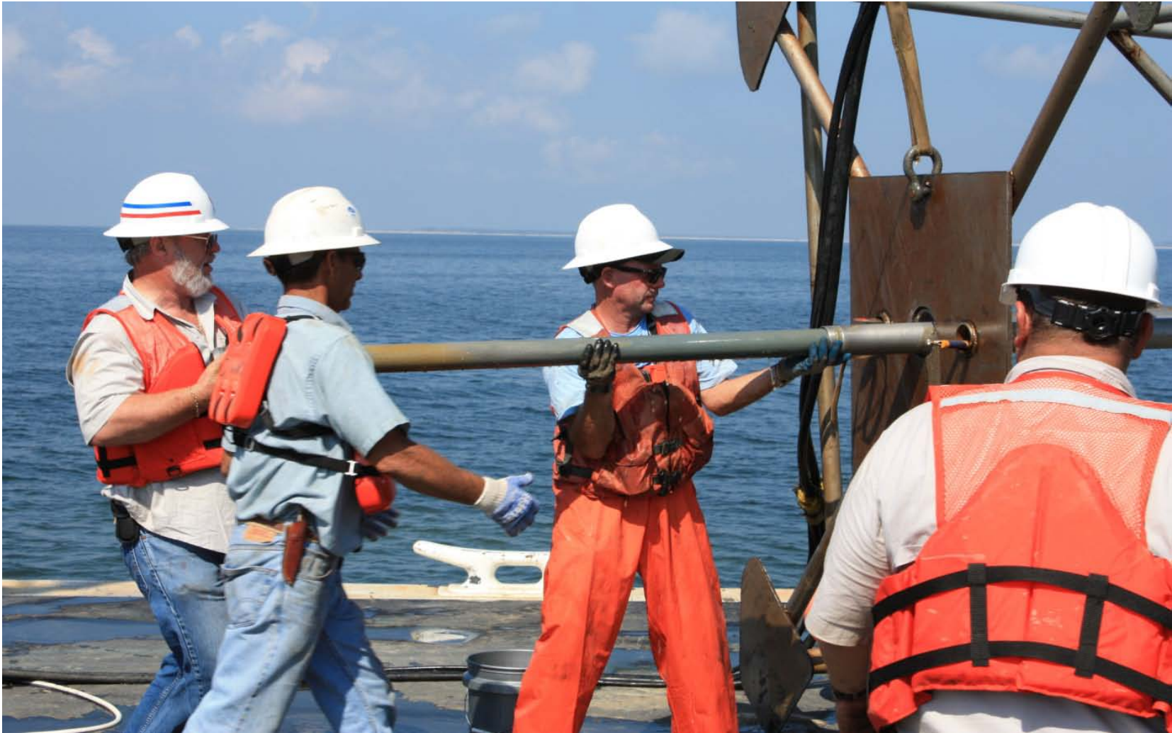
Figure 5.1.3 – The inner sleeve of the VibraCore containing the sediment sample is removed
