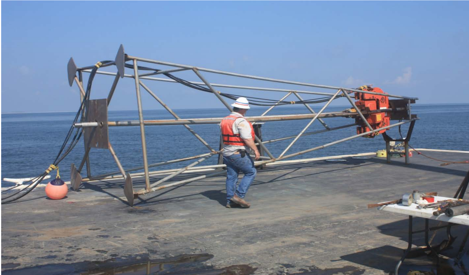
Figure 5.1.1 – VibraCore unit on the deck of the vessel. The unit is lifted from the deck by a crane and lowered to the bottom.
