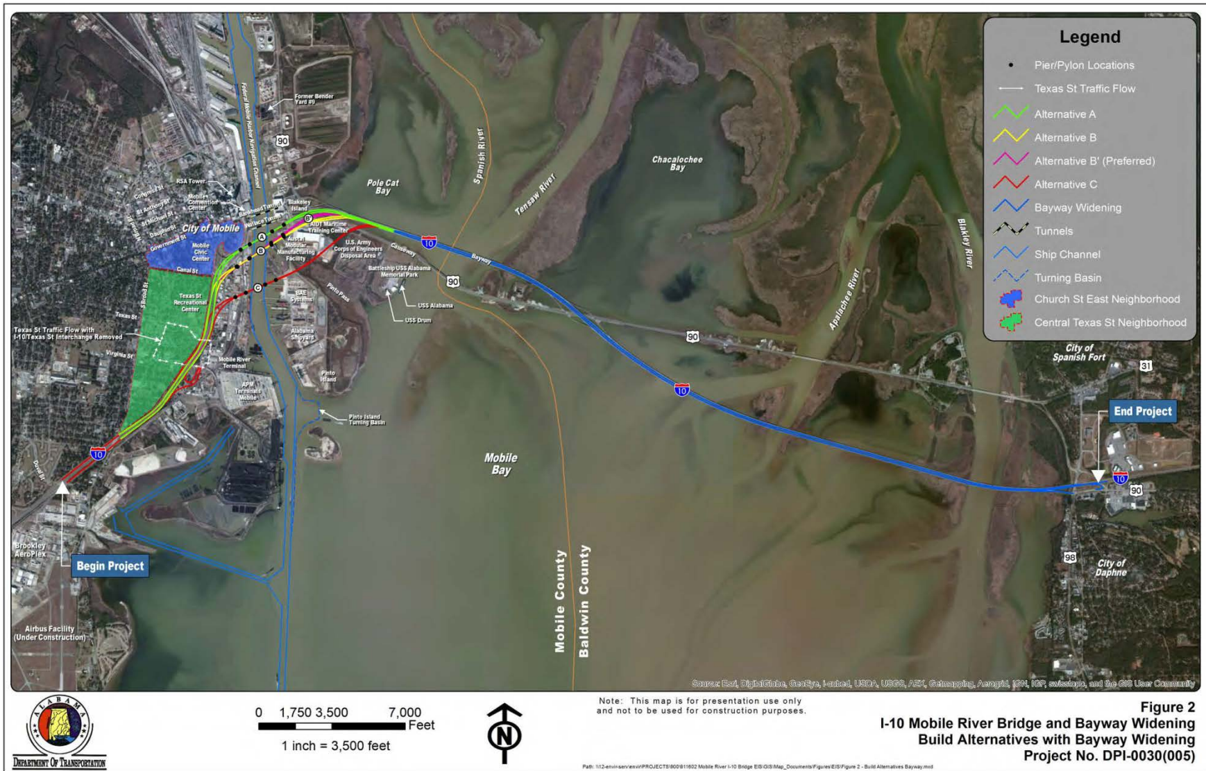
Figure 4-8. The four alternatives for the I-10 Bridge and Bayway widening project from the Draft EIS
