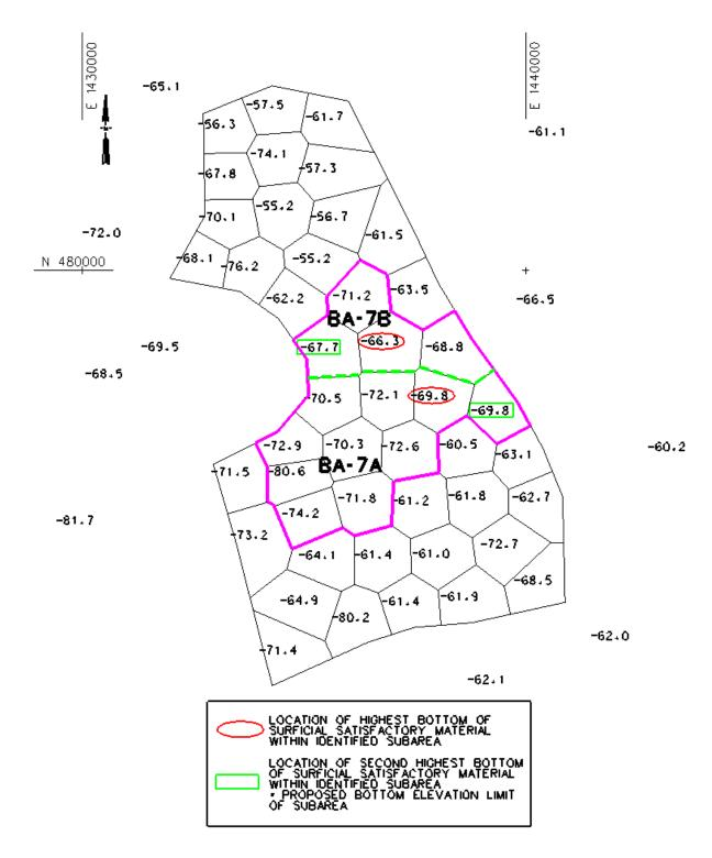
Figure A-2-9. Bottom Elevation of Satisfactory Surficial Material at BA-7
