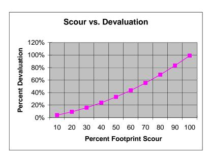
Derivation of Pecentage Devaluations for Commercial Beach Front Properties onDeep Pile Foundations caused by Foundation Undercutting Buildings from 4 to 10 stories (Computed on 4 story)
