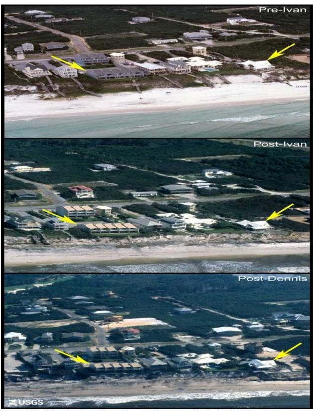
Coastal Bluff Erosion Near Town Homes: Seagrove, FL: During Hurricane Ivan, vegetation was removed from the steep bluff face. The bluff was eroded landward during Hurricane Dennis threatening structures near the bluff edge.
