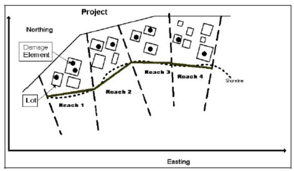
FIGURE 3. BEACH-fx SCHEMATIZATION OF STUDY AREA
