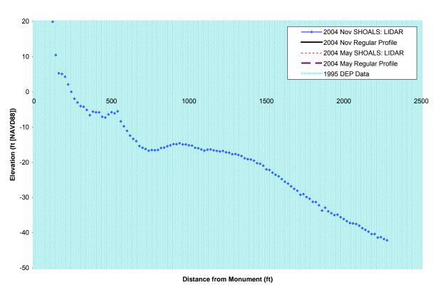
Figure A-1-20. Comparison of Recent Profile Data at R-1
