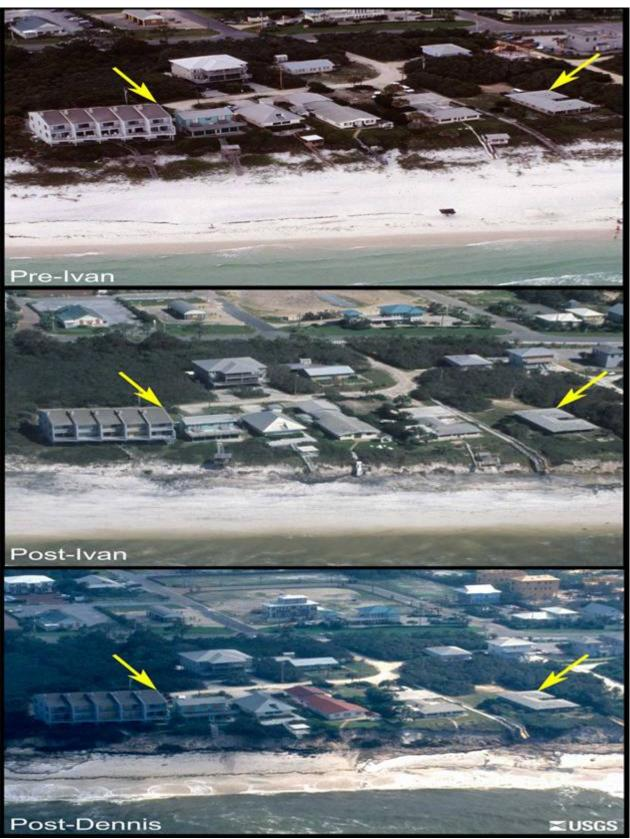
Coastal Bluff Erosion Near Homes, Seagrove, FL: During Hurricane Ivan, coastal erosion at the base of the bluff destroyed stairways. Bluff erosion continued during Hurricane Dennis.
