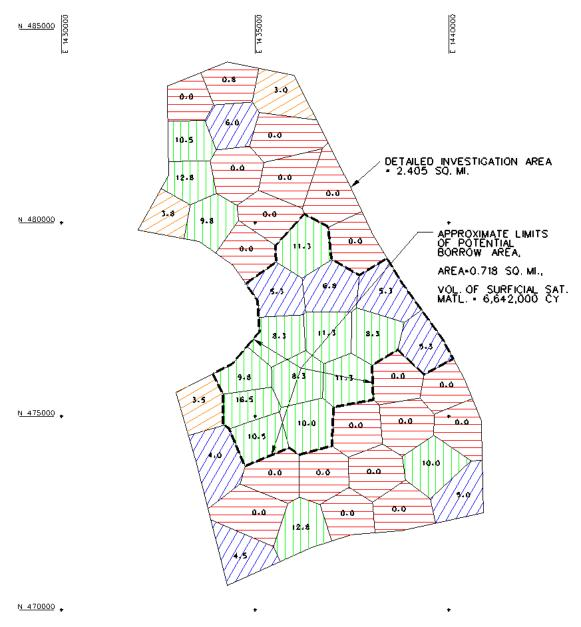
Figure A-2-6. Thickness of Surficial Satisfactory Material at BA-7
