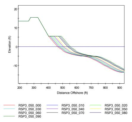
Figure A-1-56. Example SBEACH Dune and Berm Configurations for SRD
