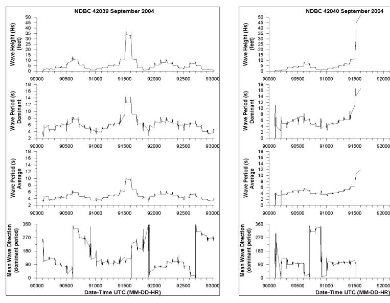
Figure A-1-43. NDBC Buoy 42039 and 42040 Offshore Wave Data - Hurricane Ivan
