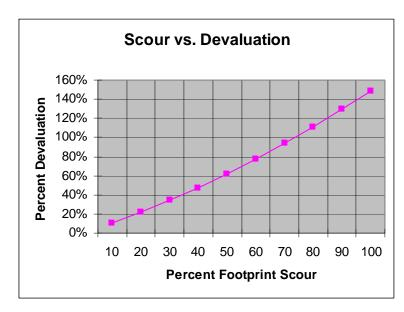
Derivation of Pecentage Devaluations for Commercial Beach Front Properties on Deep Pile Foundations caused by Foundation Undercutting
