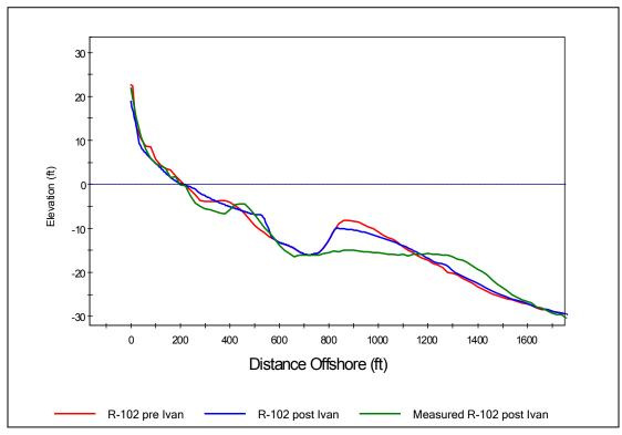
Figure A-1-47. SBEACH Calibration Profile R-102
