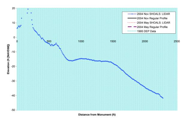
Figure A-1-23. Comparison of Recent Profile Data at R-97
