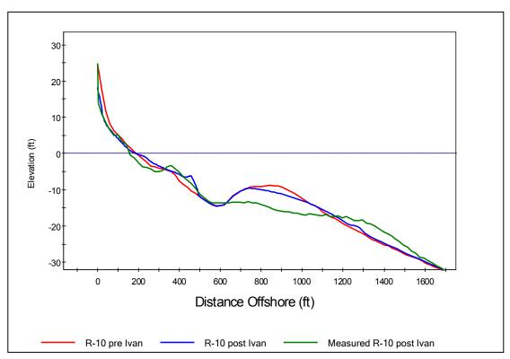
Figure A-1-45. SBEACH Calibration Profile R-10
