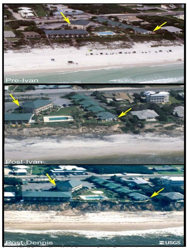
Coastal Bluff Erosion Near Hotel, Seagrove Beach, FL: Vegetation was removed from the bluff face by Hurricane Ivan. At the left center of the post-Dennis image, a pile of sand and debris is seen at the foot of the bluff.
