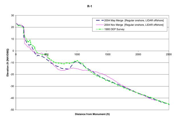
Figure A-1-22. Comparison of Merged Profile Data at R-1
