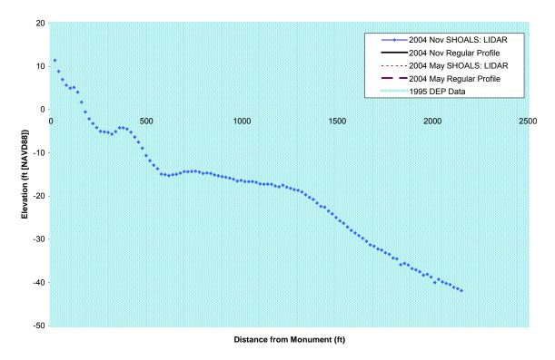
Figure A-1-21. Comparison of Recent Profile Data at R-21
