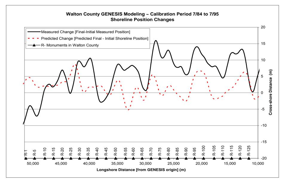
Figure A-1-33. MEASURED vs. GENESIS Predicted Shoreline Change: Calibration Period (7/84 TO 7/95) With K₁=0.13, K₂=0.1
