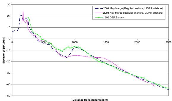
Figure A-1-25. Comparison of Merged Profile Data at R-97
