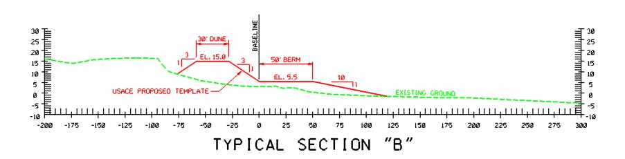
FIGURE B-6. TYPICAL PROJECT SECTIONS TO BE CONSTRUCTED
