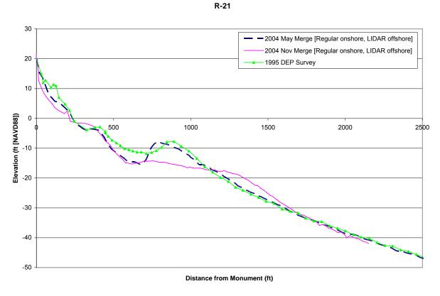
Figure A-1-24. Comparison of Merged Profile Data at R-21
