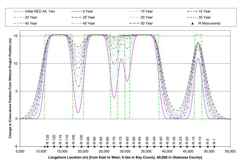
Figure A-1-38. GENESIS Predicted Shoreline Positions - Future With-Project Modeling NED Plan
