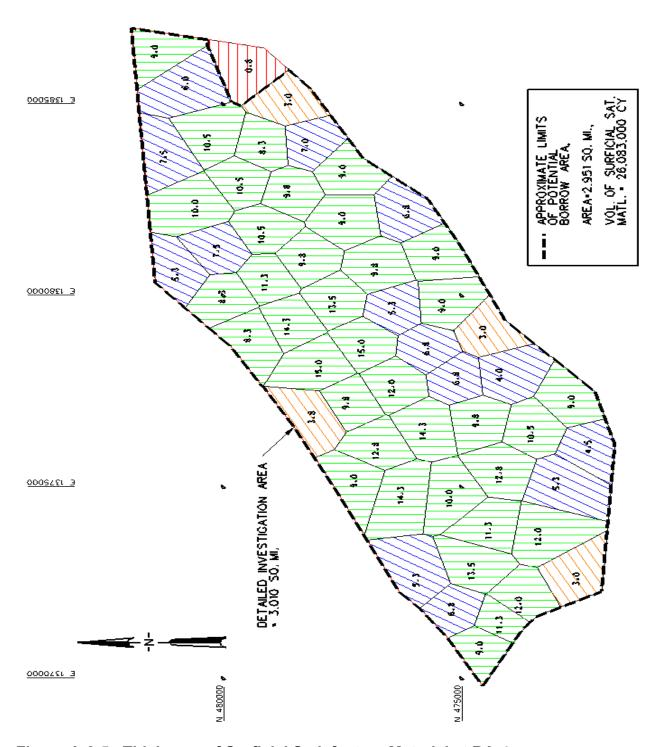
Figure A-2-5. Thickness of Surficial Satisfactory Material at BA-4
