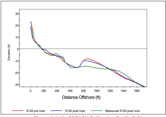
Figure A-1-46. SBEACH Calibration Profile R-50
