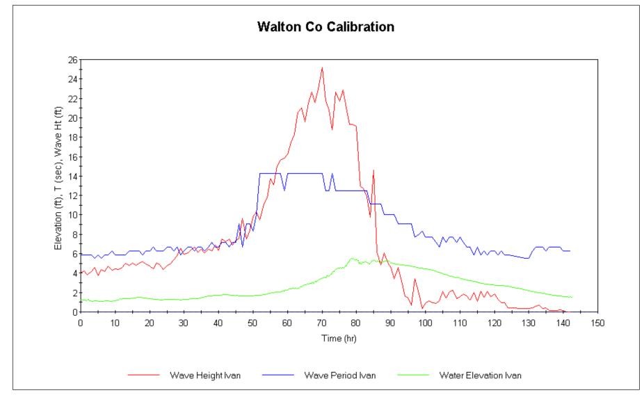
Figure A-1-44. Environmental Forcing For SBEACH Calibration (Hurricane Ivan: 13 September Through 19 September 2004)
