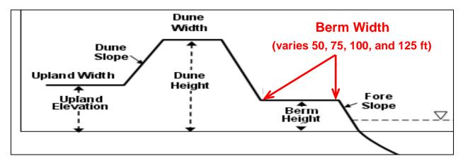
FIGURE 9. BEACH PROFILE SHOWING VARYING WIDTH OF BERM
