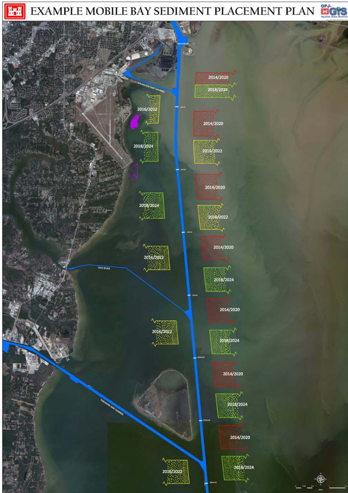
Figure 3. Example of the Strategic Sediment Placement Plan utilizing pre-established open bay placement areas.
