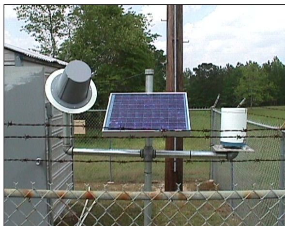
Figure 5-2. Typical Field Installation of a Precipitation Gage
