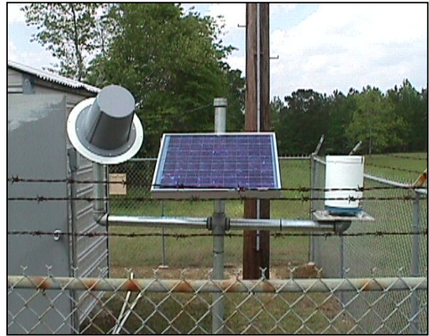
Figure 5-2. Typical Field Installation of a Precipitation Gage
