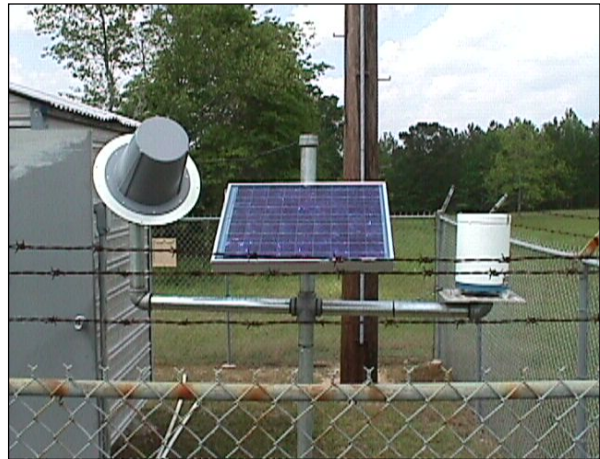
Figure 5-2. Typical Field Installation of a Precipitation Gage
