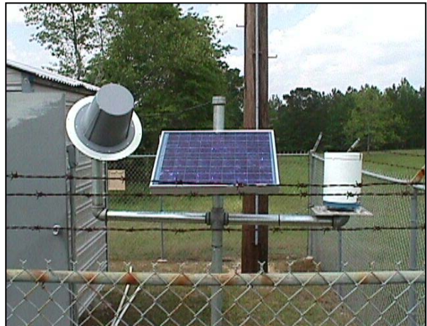
Figure 5-2. Typical Field Installation of a Precipitation Gage
