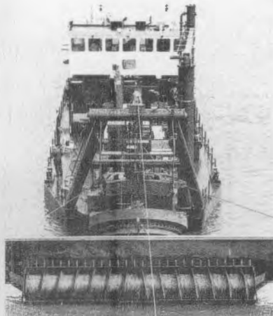
The encapsulated bucket dredger (above) and the auger dredger (left) are two examples of specially designed environmental dredging equipment.
